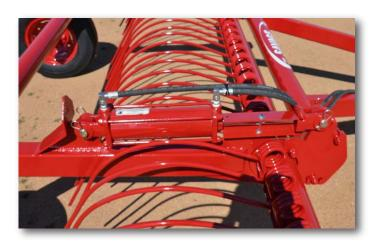
All Savage rakes feature hydraulically controlled tines enabling the operator to adjust for the terrain and type of debris. Tines are very simple to replace and can be replaced individually as needed.
